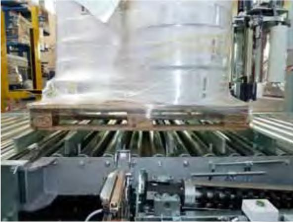
The pallet lifter raises the pallet during the wrapping process to ensure proper placement of film or rope on a shorter pallet. You can wrap down to the very bottom or even under the pallet, depending on your needs.
