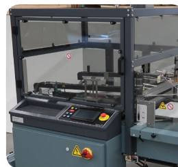
New Guarding featuring Dual Monitored Safety Circuit
